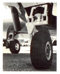
Rugged Mooney gear has no fancy hydraulics or oleos to run up shop bills. Positive-action energy-absorbing electric gear retracts or extends in just seconds.
